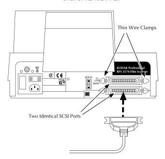
4. Attach the SCSI terminator (supplied with the Scanner) to the empty SCSI port on the Scanner, seat the terminator firmly, and pinch the thin wire clamps shut.
